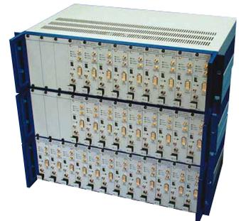
30-channel controller consisting of 3 E-500.621 chassis, each of which can accommodate up to 12 E-621 modules
