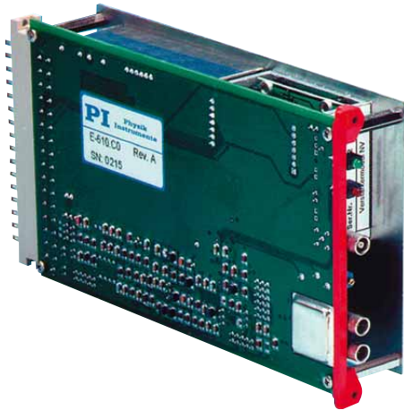
E-610 Single-channel OEM module with optional position servo control
