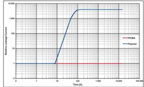
PICMA<sup>®</sup> piezo actuators (bottom curve) compared with conventional multilayer actuators with polymer insulation (top curve). PICMA<sup>®</sup> actuators are not affected by the high-humidity test conditions. Conventional piezo actuators exhibit increased leakage current after only a few hours. Leakage current is an indicator quality and expected lifetime.
