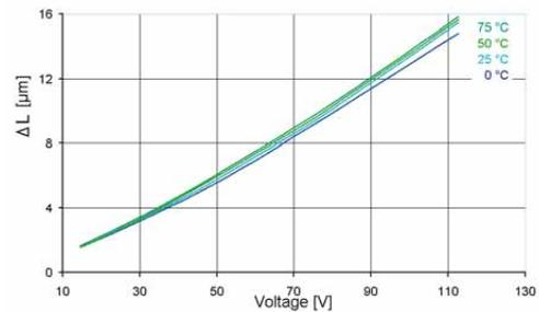
The displacement of PICMA<sup>®</sup> actuators exhibits very low temperature dependence. This, in combination with their low heat generation, makes PICMA<sup>®</sup> actuators optimal for dynamic operation
