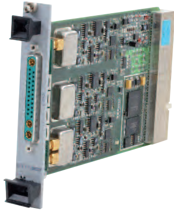
E-711.SC3H sensor module for capacitive dual-plate sensors with nanometer resolution
