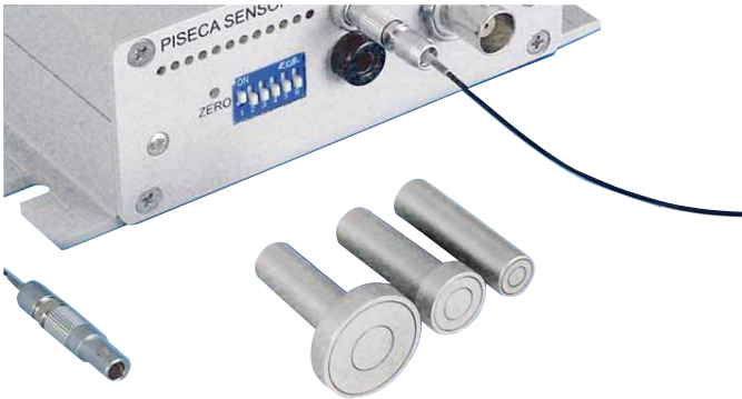
PISeca high-precision capacitive sensor probes with E-852 signal conditioner electronics. Sensor probes (from left): D-510.101 with 100 \mu\text{m} , D-510.051 with 50 \mu\text{m} , D-510.021 with 20 \mu\text{m} nominal measurement range
