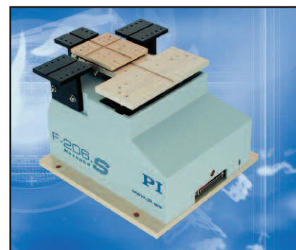
Figure 10. Six-axis precision hexapods are based on parallel-kinematic flexure designs and provide long travel motion in all six degrees of freedom with a user-definable pivot point.
