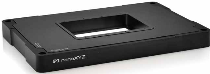
The low profile of 20 mm and special design to allow for a full slide to be mounted at the bottom set Plnano™ piezo microscope stages apart. The Plnano™ Trak version shown above is optimized for extremely fast motion and provides sub-nanometer resolution in up to three axes
