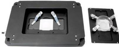
Plnano™ Z piezo slide scanner / fast focusing stage for high resolution microscopy
