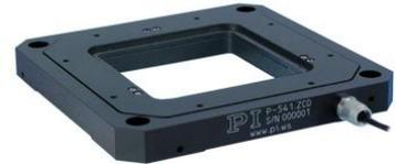
P-541 piezo Z-stage & Z-tip/tilt stage. Sub-nanometer resolution, travel to 100µm. Very low profile (16.5mm) and large 80x80mm aperture
