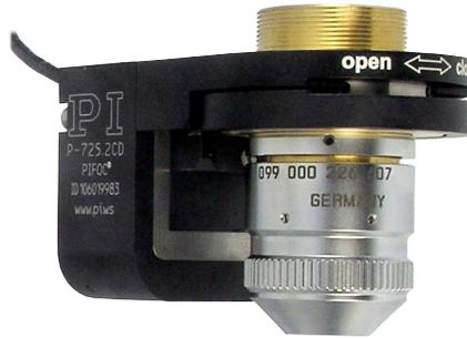
Instead of moving the sample, it is also possible to move the objective. PIFOC® Objective Scanner offers travel ranges to 1000 µm with nanometer resolution and response times in the millisecond range
