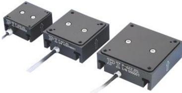
P-62x.Z PIHera® family of nano-precision elevation stages. Z-travel 50 to 400µm. Piezo-flexure drive, capacitive feedback
