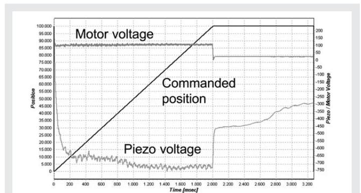
PI hybrid servo-controller output during a positioning command. The controller reads the system position off a high-resolution encoder and actuates both the motor and piezoelectric actuator at the same time giving a system with the advantages of both drives.
