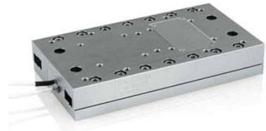
N-664 High Resolution Linear Translation Stage with PiezoWalk® Linear Motor. 0.5 Nanometer Linear Encoder Resolution, 2nm minimum incremental motion
