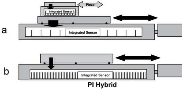
Different types of combined motorized and piezo positioning systems:
