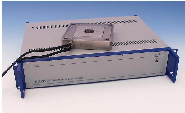
Fig 11a. State-of-the-art 6 axis digital controller and custom Super Invar 6D piezo scanning stage (parallel-kinematics mechanics and parallel motion metrology).
