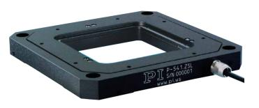
P-541 series nanopositioning Z-stages and Z-tip/tilt stages offer travel ranges of 100 μm with sub-nanometer resolution. They feature a very low profile of 16.5 mm and a large 80 x 80 mm aperture. Versions with strain gauge and capacitive position feedback sensors are available
