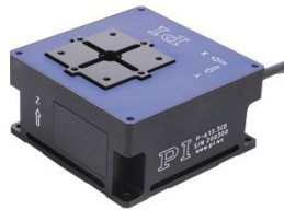
P-615 Long-Travel NanoCube® XYZ nanostage with aperture. Up to 420μm travel, capacitive feedback
