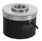
P-726 High-dynamics  $PIFOC^{\odot}$  objective scanner for heavy, high NA microscope objectives, 100  $\mu$ m travel range capacitive feedback.
