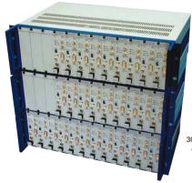
30-channel controller consisting of 3 E-500.621 chassis, each of which can accomodate up to 12 E-621 modules
