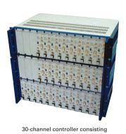
of 3 E-500.621 chassis, each of which can accomodate up to 12 E-621 modules
