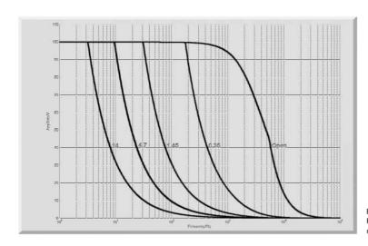
E-616: operating limits with various PZT loads (open-loop), capacitance is measured in  $\mu\text{F}$
