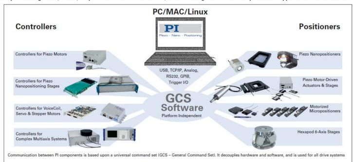
Communication between PI components is based upon a universal command set (GCS – General Command Set). It decouples hardware and software, and is used for all drive systems
