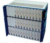
Multi-channel controller consisting of 3 E-500.621 chassis and 30 E-621 modules
