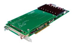
E-761 Digital Piezo Controller PCI-Board, 3 Channel
